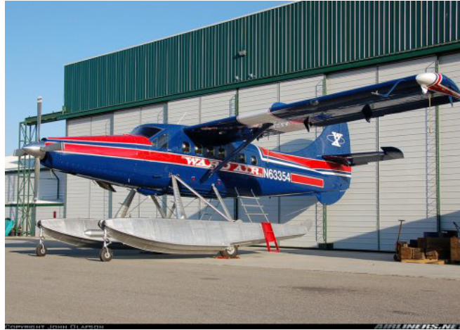
Turbo Otter with Garrett TPE331-10 engine and 4 blade propeller
